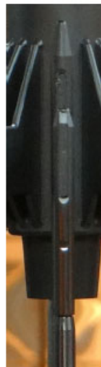
Pinned EP-RCCA rodlet connection
